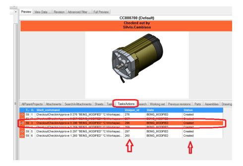
In order to keep those tabs as clear as possible, successfully completed tasks are removed from this tabs because the user can see directly on the tree from the status of the involved documents.
