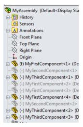
where the MyFirstComponent has <u>some</u> suppressed instances, the MySecondComponent has <u>all</u> its instances being suppressed, and the MyThirdComponent has <u>no</u> suppressed instance, its Tree is now displayed <u>everywhere</u> as:
