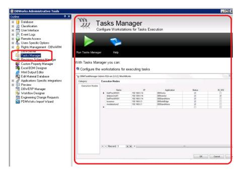
Launching this tool, you will be able to configure the executing nodes, specifying for each of it the name, its IP, the application running on it (which will be used to run tasks), whether it's enabled or not (STATUS), if it's a general working server or a specific user machine (IS\_WS):
